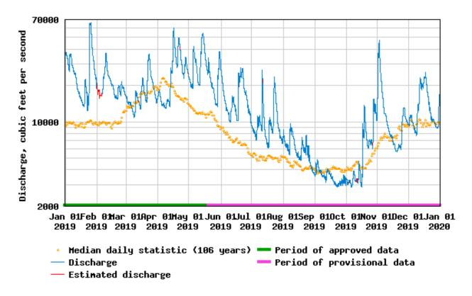
**Figure 2.** USGS discharge from Delaware River at Trenton (USGS station 01463500) during 2019. Freshwater inflow was well above the long-term median for much of the year. These conditions reduced salinity over the oyster beds as shown in figures 3 and 4 below.
