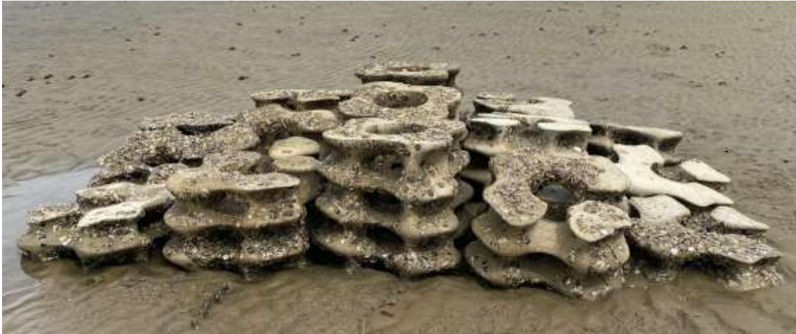
Figure 2-10. Oyster Growth Displayed on Testing of Reefense Modules
