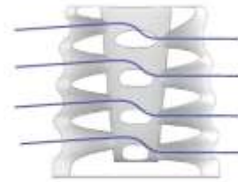
Holes on opposite sides adjusted to slow water movement. However, solid base is maintained in pouring process.
