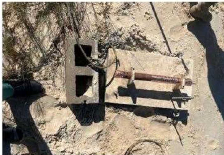
Figure 3. Water Quality Sonde Equipment and Example Deployment Method. Insitu Aquatroll 500 series water quality sondes will be attached to concrete block base and further secured using standard construction cinder blocks.
