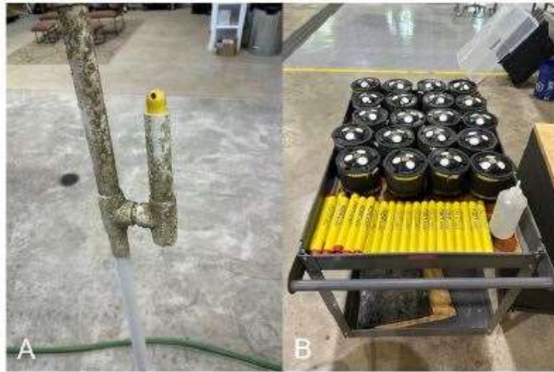
Figure 2. Wave Gauge and ADCP Equipment and Example Deployment Methods. RBR soloD wave gauges (yellow instruments) will be deployed within 1.5 inch PVC pipes forced into bed sediments. A zip tie secures the instrument to the pipe through a hole at the top of the RBR (A). Nortek Signature 1000 ADCPs (black instruments) are secured to a 6 inch PVC pipe pushed into bed sediments using a rubber pipe coupler (B).
