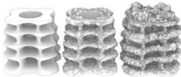
Figure 2-9. Conceptual Oyster Growth on a Reefense Module
